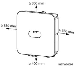
• When installing multiple inverters, install them in horizontal mode if sufficient space is available and install them in triangle mode if no sufficient space is available. Stacked installation is not recommended.
