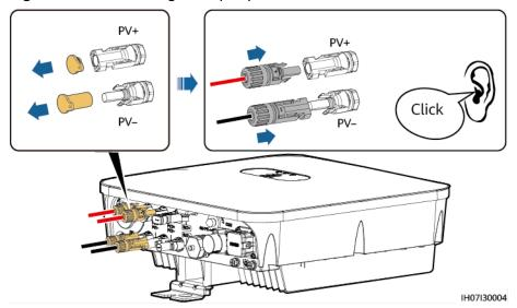
Figure 5-15 Connecting DC input power cables
