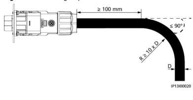
Figure 5-11 Cabling requirements
