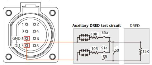
Figure 7-12 Wiring diagram for the DRM function
