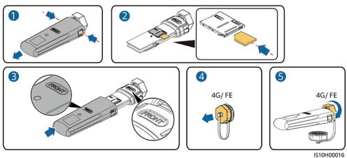
Figure 5-4 Installing a 4G Smart Dongle
