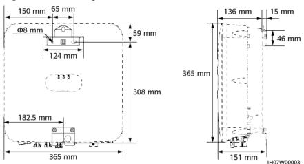
Figure 4-7 Mounting bracket dimensions
