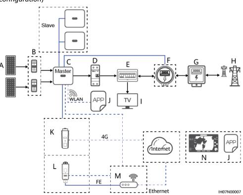
**Figure 2-3** Inverter cascading scenario (dashed boxes indicate optional configuration)
