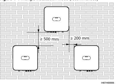
Figure 4-4 Triangle installation mode (recommended)
