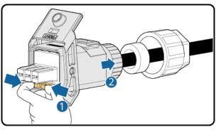
Figure 5-12 Removing a plug insert
