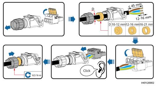
Figure 5-7 Assembling an AC connector (three-core wire)
