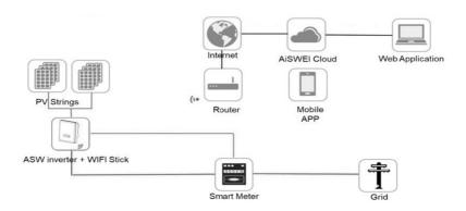
The smart meter should support the MODBUS protocol with a baud rate of 9600 and address set 1. Smart meter as above SDM630-Modbus connecting method and seting baud rate method for modbus please refer to it's user manual.
