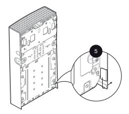
Pull out the lower portion of the cover in order to unlock the angular tabs and move it away from the wall slightly.
