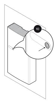
Apply AC power to the IQ Battery 5P circuits. Turn ON the DC control switch. A green LED will glow around the control switch. IQ Battery 5P is ready for commissioning.
