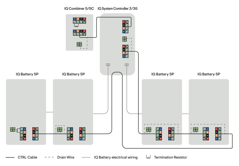
**NOTE:** Total length of CTRL wiring across the system cannot exceed 250 feet to ensure the system operates as per specifications.
