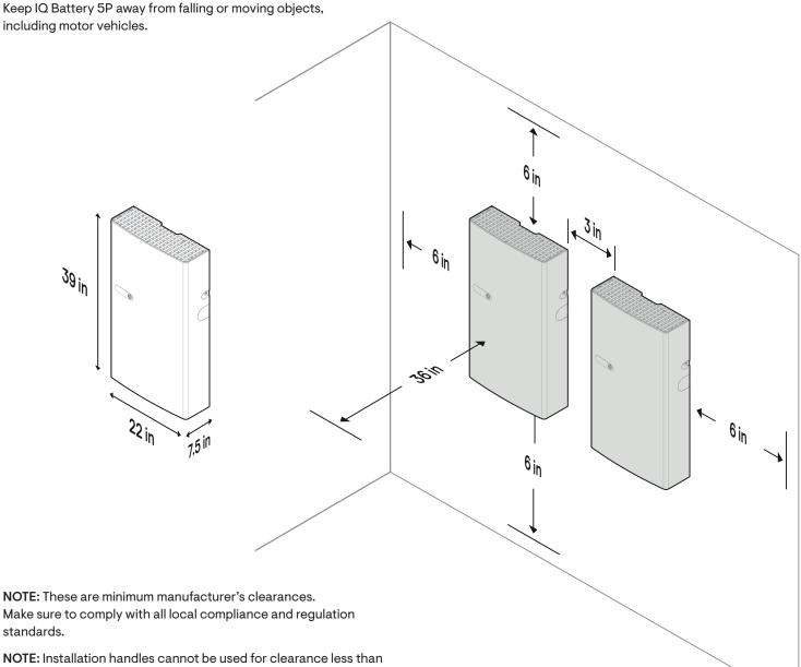
5.5". Installers need to consider adjusting the distance between batteries based on the cable bending radius.
