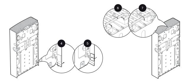
Before releasing, pull out the lower edges while sliding in the cover and make sure the tabs are locked to the back plate. Push in the top portion of the cover as shown and make sure that the cover is locked in place.
