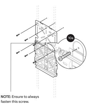
Fasten the top shield using the mounting holes. Use a minimum of six screws for single stud and dual stud mounting to fasten the top shield to the wall. Use standard screws only (head thickness <5 mm). Finally, fully tighten the grounding screws (torque to 1.5 N m/13.28 lb-in).
