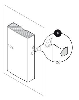
After installing the cover, the conduit cover should be installed to cover the opening in the IQ Battery 5P cover on the side.
