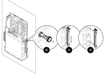
To remove the installation handles, pull the plunger outward to unlock them. Then, slide the handle down and pull it away from the unit to remove it.
