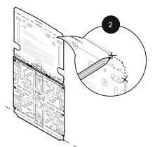
Starting at the installation position closest to the power source, mark a level line on the wall as a guide.
