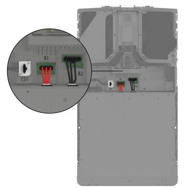
NOTE: Connect CS1 at last to avoid damage to the wiring cover
