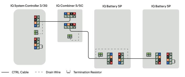
**NOTE:** Total length of CTRL wiring across the system cannot exceed 250 feet to ensure the system operates as per specifications.
