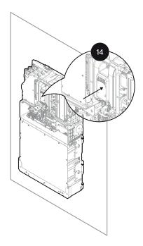
Push against the wiring cover and hold the IQ Battery 5P top section as close to the wall as possible.
