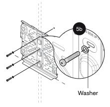
Position the bottom mounting bracket on the wall and fasten it using the mounting slots.
