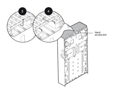
Using the hand access slot, pull the top plastic grill slightly, as shown in step 3.
