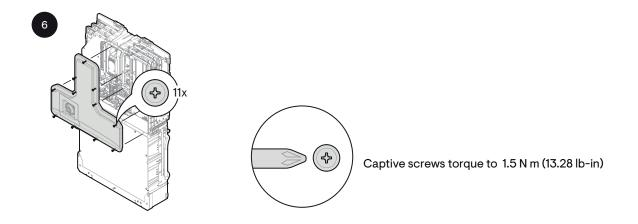
Open the front wiring cover by unfastening the 11 captive screws from the wiring cover. Use an electric drive; do not use impact drives/impact drills.
