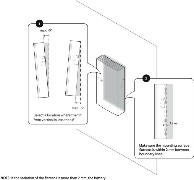
NOTE: If the variation of the flatness is more than 2 mm, the battery might not properly sit on the bottom mounting bracket through keyholes. Use spacers if the variation is more than 2 mm.
