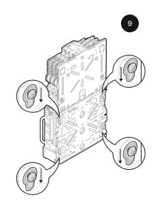
Bring the IQ Battery 5P unit to the already mounted bottom mounting bracket.
