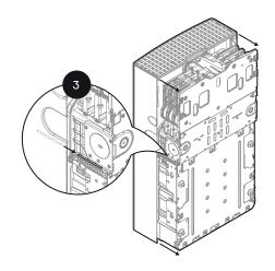
Slide on the IQ Battery 5P covers in the indicated direction such that the tab of the cover in the highlighted region rests and slides on the latch in the IQ Battery 5P chassis.
