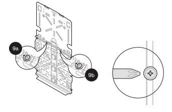
Partially tighten the top shield to the bottom mounting bracket at the ground contact flange.
