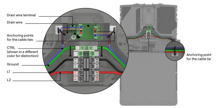
$\Delta$  Make sure the drain wires do not come in contact with any live connection.
