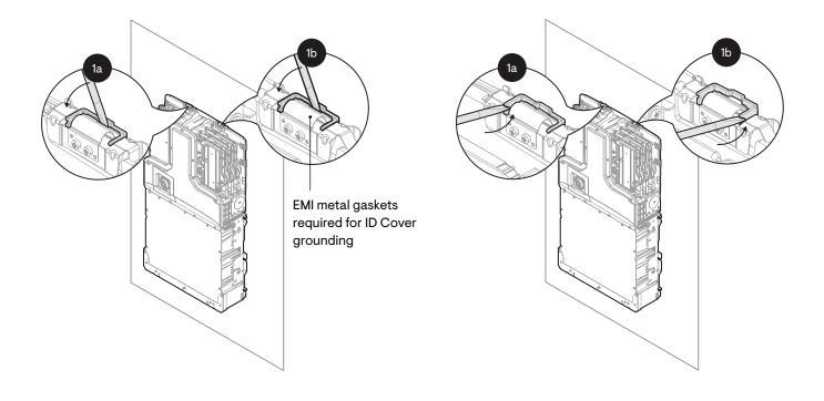
Disengaging of the anchor clip can be done by lifting it up using a flathead screwdriver or nose plier. Installers need to carefully insert the tool at the back slot, as shown below, and pull the clip upwards.
