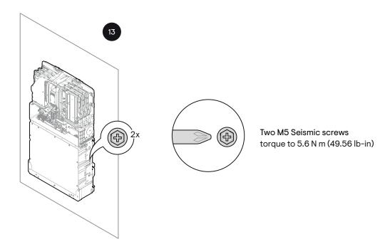
Secure the battery unit on the bottom mounting bracket using two M5 Seismic screws. This is required to comply with seismic requirements.
