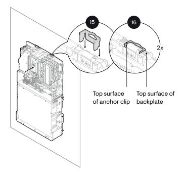
Install two anchor clips to secure the top section of the IQ Battery 5P to the wall. Slide the anchor clip downwards until the top surface of the clip coincides with the top surface of the IQ Battery 5P backplate. This ensures no obstructions during the IQ Battery 5P cover installation.
