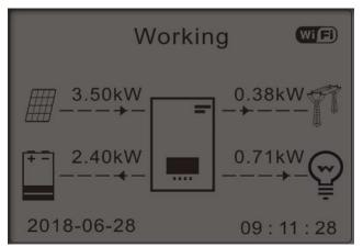
4) If PV generation < LOAD consumption, it will discharge the battery to supply power to load.
