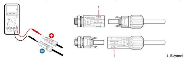
Fig. 9 Connect PV connectors
