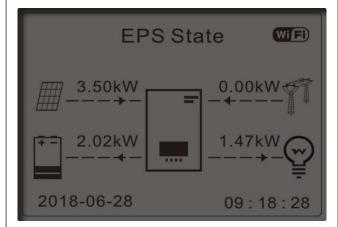
2) If PV generation = LOAD consumption, HYD-ES inverter wont' charge or discharge battery.
