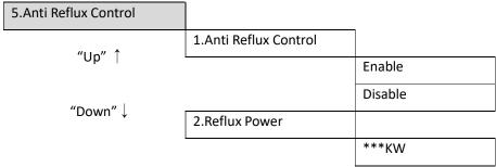
The user can enable "Anti Reflux Control" to limit the max export power to grid.
