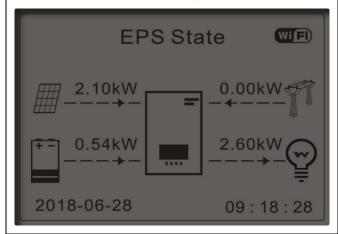
4) If PV generation is normal, but LOAD consumption=0, the surplus power will be stored in the battery.
