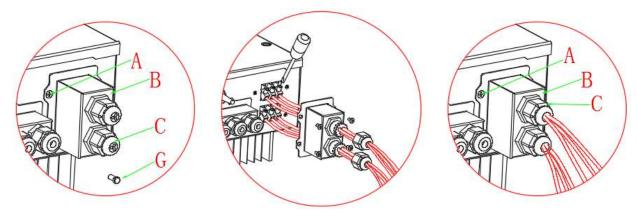
Fig. 14 Grid & Load connection
