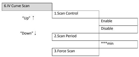
The user can enable "IV Curve Scan" (MPPT scan) to make HYD-ES inverter to find the global max power point periodically to deliver max power from a partially shaded PV array.
