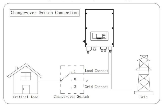
Fig. 15 Change-over Switch connections
