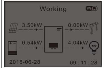
5) If PV generation + Battery < LOAD consumption, HYD-ES inverter will import power from the grid.
