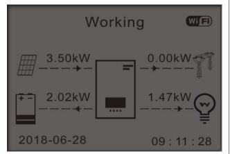
3) If the battery is full(or already at Max Charge Power), excess power will be exported to the grid.
