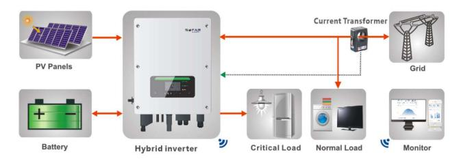
Fig. 1 HYD-ES inverter schematic diagram
