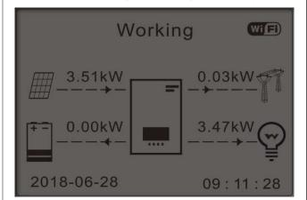
2) If PV generation > LOAD consumption, the surplus power will be stored in the battery.
