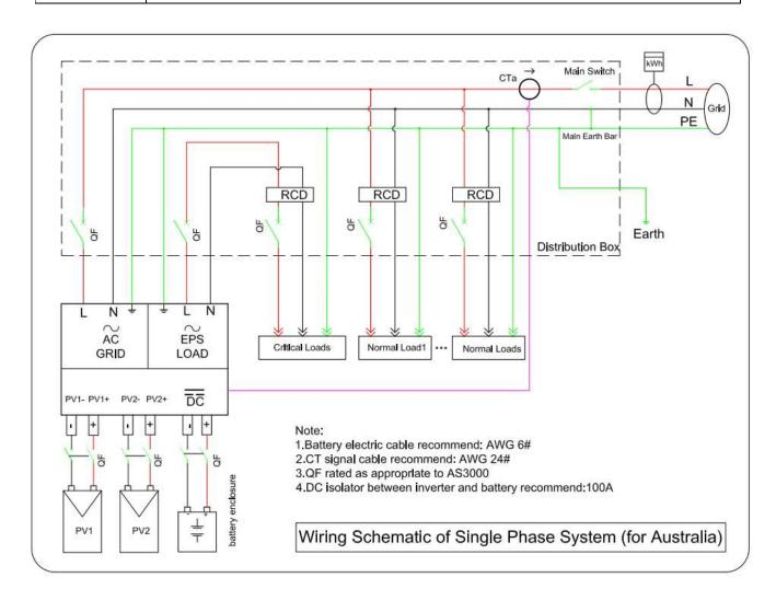
Fig. 5 Electrical connections
