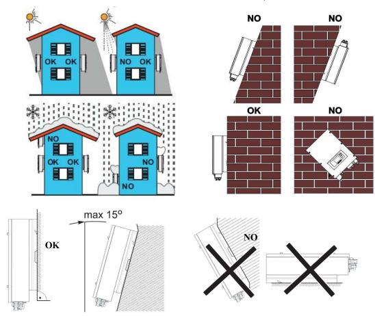
Fig. 4 Installation Position of HYD-ES inverter
