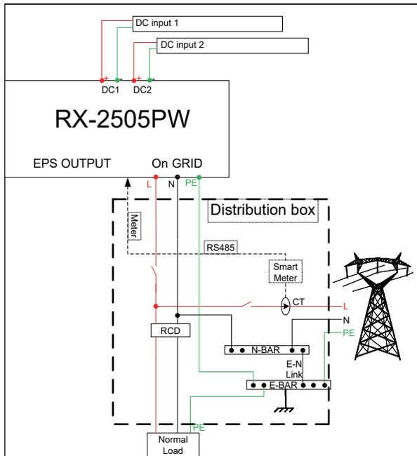
Figure 5-9 – 240V connection diagram On-grid only
