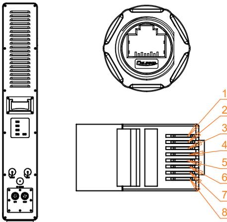
Figure 5-15 - DRM RJ45 pins
