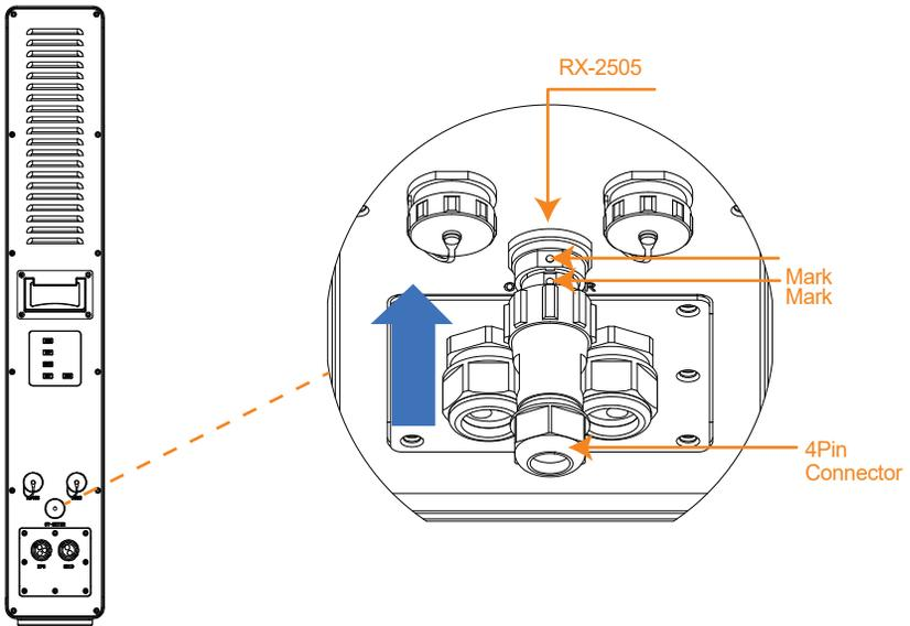
*Figure 5-10 – CT connector insertion with white guide marks*
