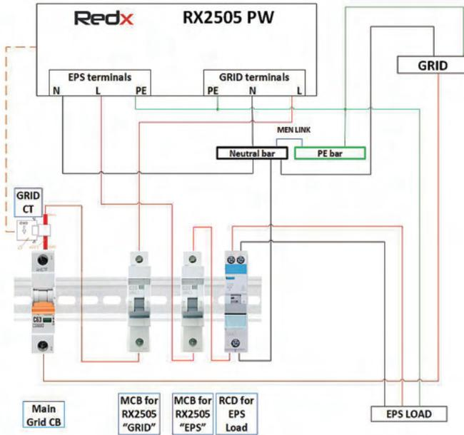
Figure 5-8 - Example switchboard installation NEUTRALS SEPARATE
