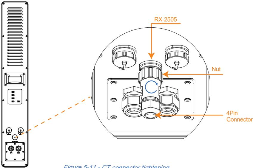
*Figure 5-11 - CT connector tightening*
