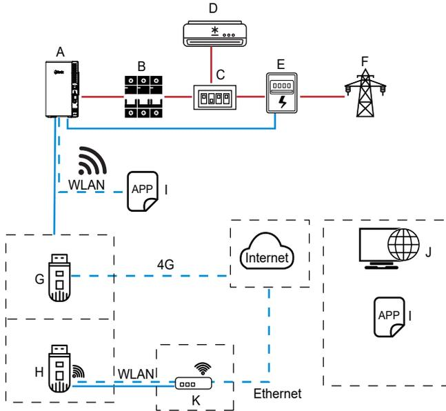
Figure 4-1 – Battery system connections topology
