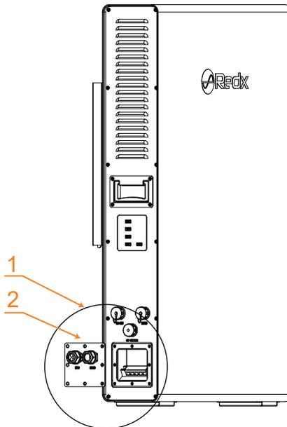
*Figure 5-1 – Battery 240V terminals and covers*
